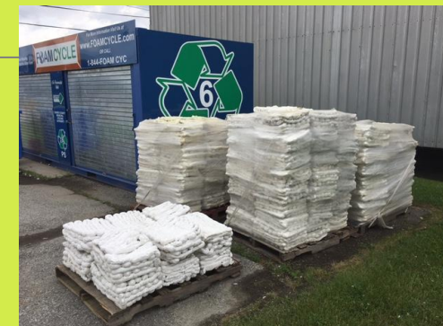
Step 3 - Aggregate Stockpile Densified "Ingots"
